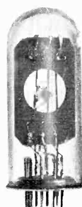
Plessey matrix store using a single barium titanate crystal
