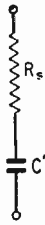
Fig. 2. This circuit is equivalent to Fig. 1 at any particular frequency, if the values are correctly chosen for that frequency.
